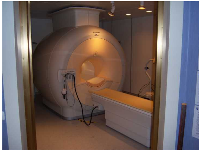
Figure 1. A 1.5 T magnetic resonance imaging scanner.
