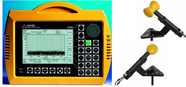
Figure 3. Narda SRM-3000 analyser and single-axis probes for the electric field, 3531/02 (top), and for the magnetic field, 3551/01 (bottom).
