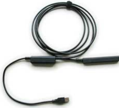
Figure 4. Metrolab THM-1176 static magnetic field probe.
