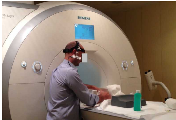
Figure 5. Measurement of the perceived magnetic flux density (pMFD) in case of movement in the static magnetic field, during the execution of movements typical of the preparation of an MRI examination.
