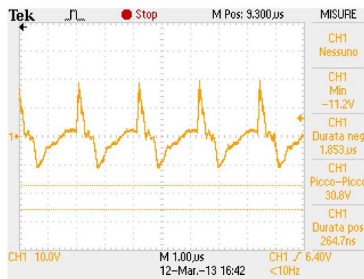
Figure 6. Alsa Excell MCDS electrosurgical unit, cutting mode, voltage waveform on a commonly used 500 \Omega load resistance.
